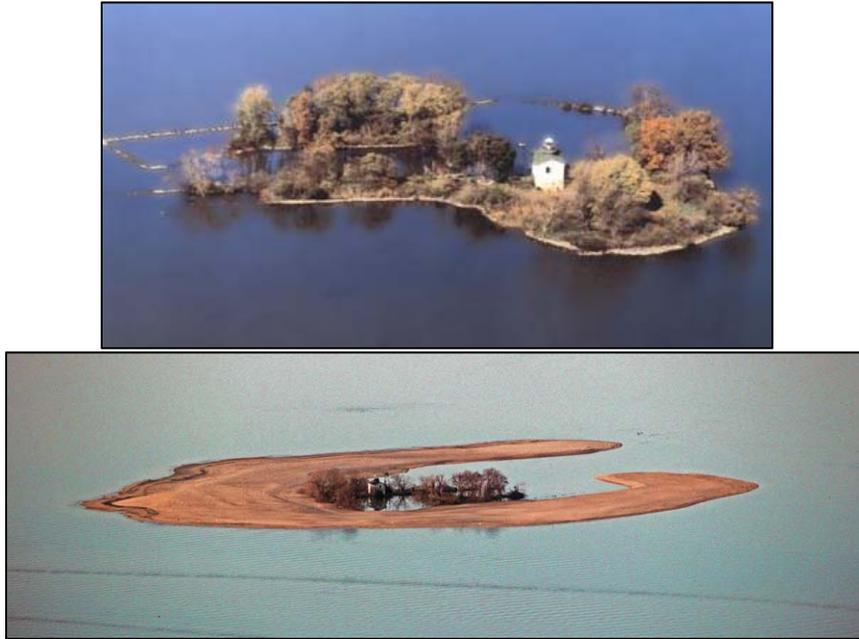
**Photo 5 Fishing Battery Island, Susquehanna Flats—Restored with the use of Dredged Material—Pre- and Post-Restoration, 2017 (USFWS Website 2019)**
